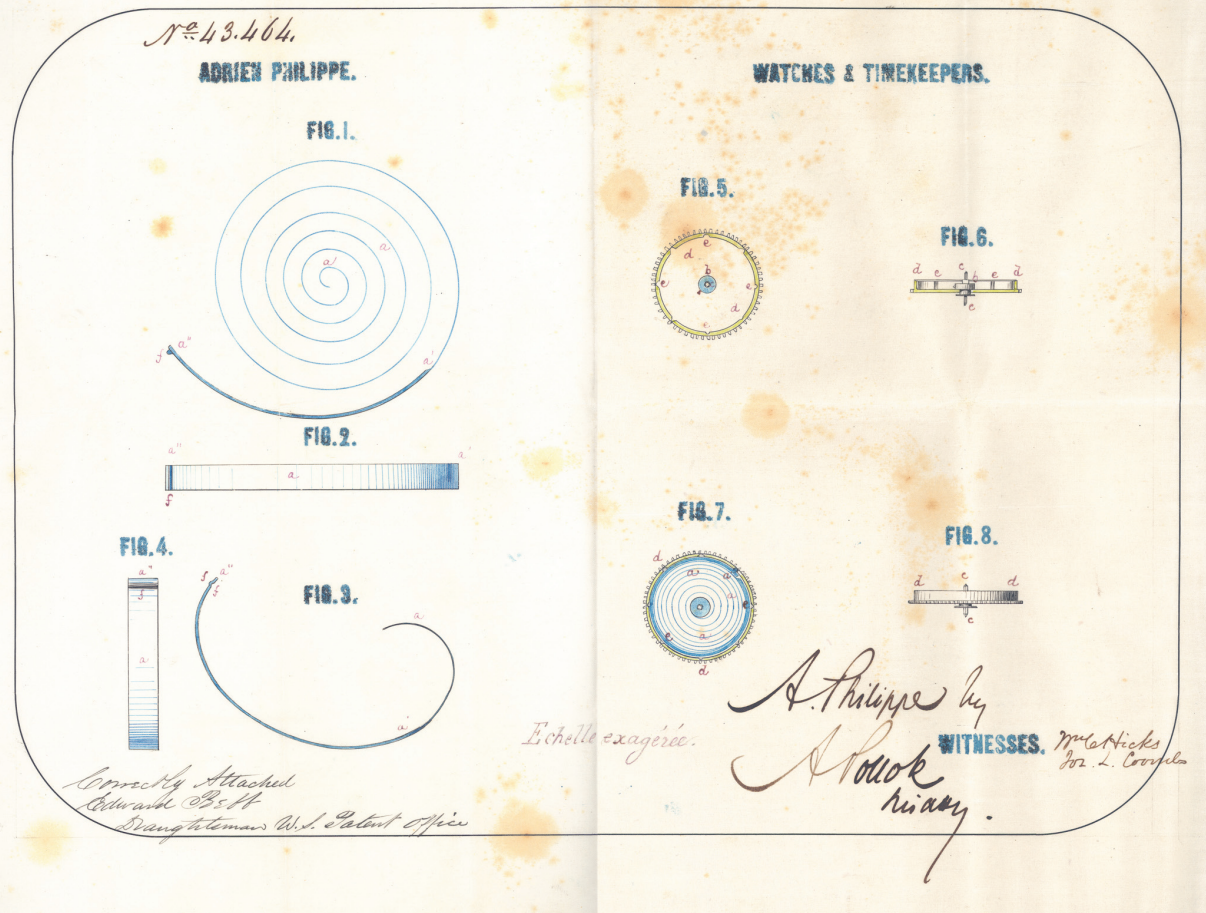
The original patent drawing for a slipping bridle mainspring by Patek Philippe
